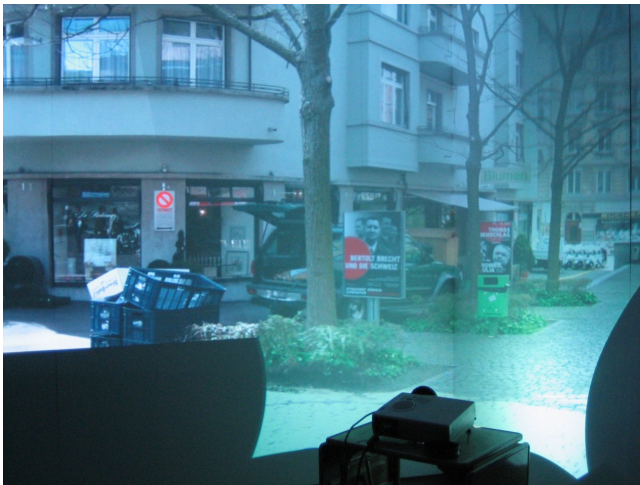
Figure 6: Display system combining a conventional projector and a fisheye-lens projector.
