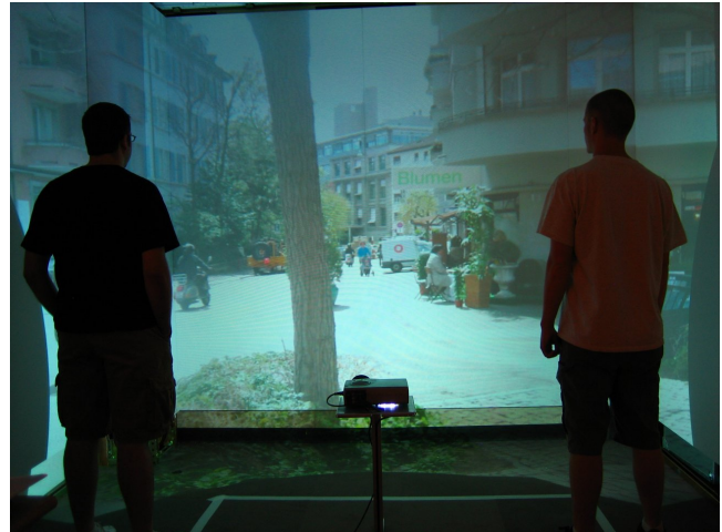
Figure 1: An immersive display built with a single fisheye projector.
