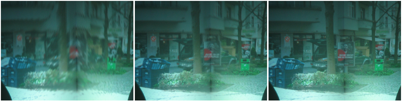
Figure 4: a) Three-pass correction for display surface geometry and fisheye distortion. b) Three-pass correction super-sampled 4x. c) Our two-pass method without super-sampling.
